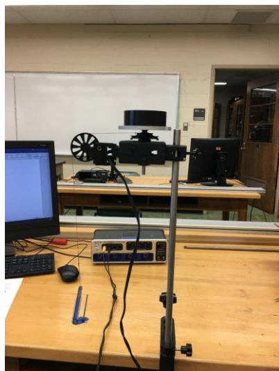
Figure 2: Measuring the Rotational Inertia of Ring and Disk
