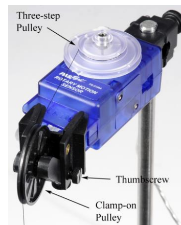
Figure 4: Adjusting Angle of Clamp-on Pulley
